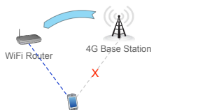
Mobile Data Offloading (Outsource cellular network to WiFi network)
